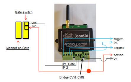
Please note that if the Gcom520 is located or mounted in a metal housing, the existing antenna must be removed and replaced with an external antenna with a SMA-RF connection.
